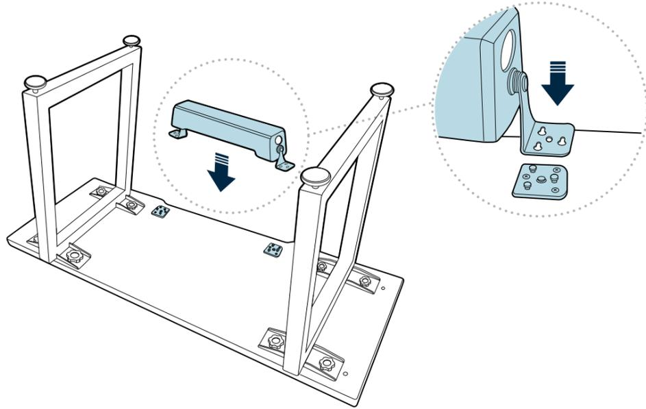
Lower the notches on each end of the cable tray over the brackets, and slide the tray (either toward the front or back of the desk) until the notches click into place.
